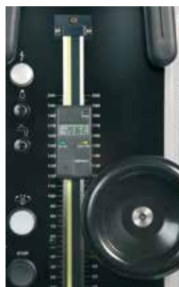
LBC Depth scale read-out system. Available for all series.
